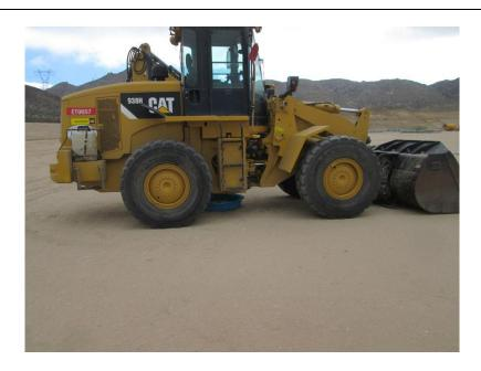
**Photo 5:** Secondary containment is observed beneath staged equipment to prevent leaks and spills in accordance with Mitigation Measure HYD-1 and the SWPPP.
